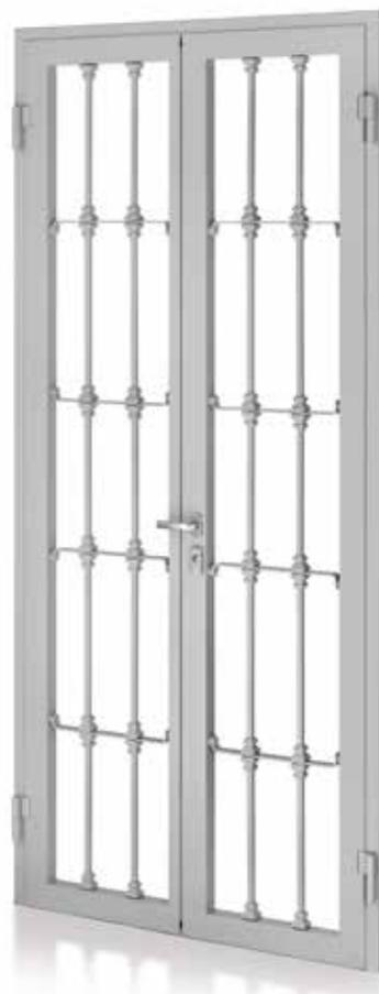
*Gate for doors built with steel-clad profile, zinc-plated and coated with weather-resistant polyester powders, frame mounted with adapters so suitable to be installed directly into the door reveal (without subframe), supplied with rubber weather stripping, multi-point lock and Yale cylinder. Made in any model.*
